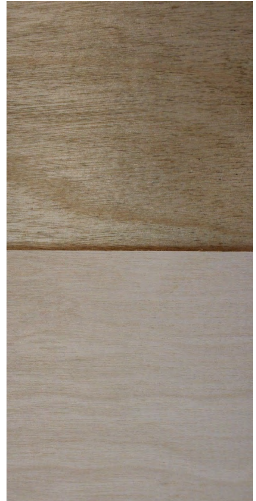
Natural Danish oil applied on birch ply (comparing with and without oil)
