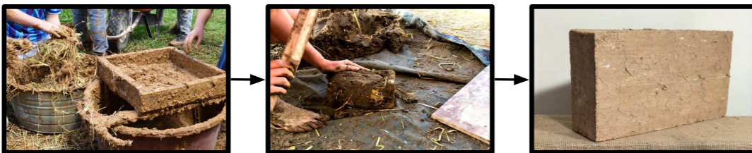
Images (above) show different stages of a cob brick creation.
