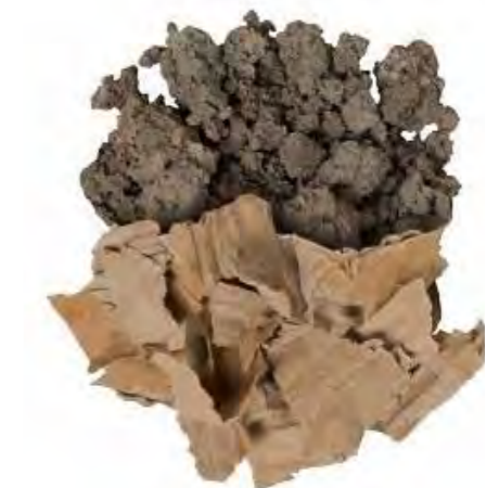
The images above show the three main stages of cellulose fibreboard making process. It starts with paper waste being shredded cellulose fibre, which is then mixed with water binder and fire retardant. Finally the mixture is compressed to form a compact solid board.
