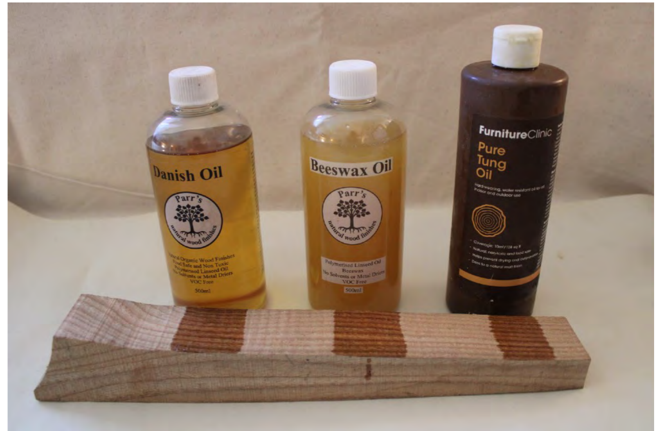
Test of different oils, (Danish oil, Beeswax Oil and pure Tung oil) on oak block
