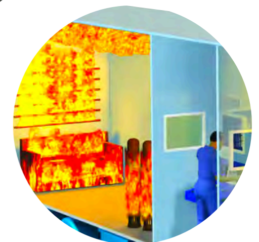
Fire simulation software can model how materials and architectures behave in fire conditions and aid in the design of a fire strategy.
