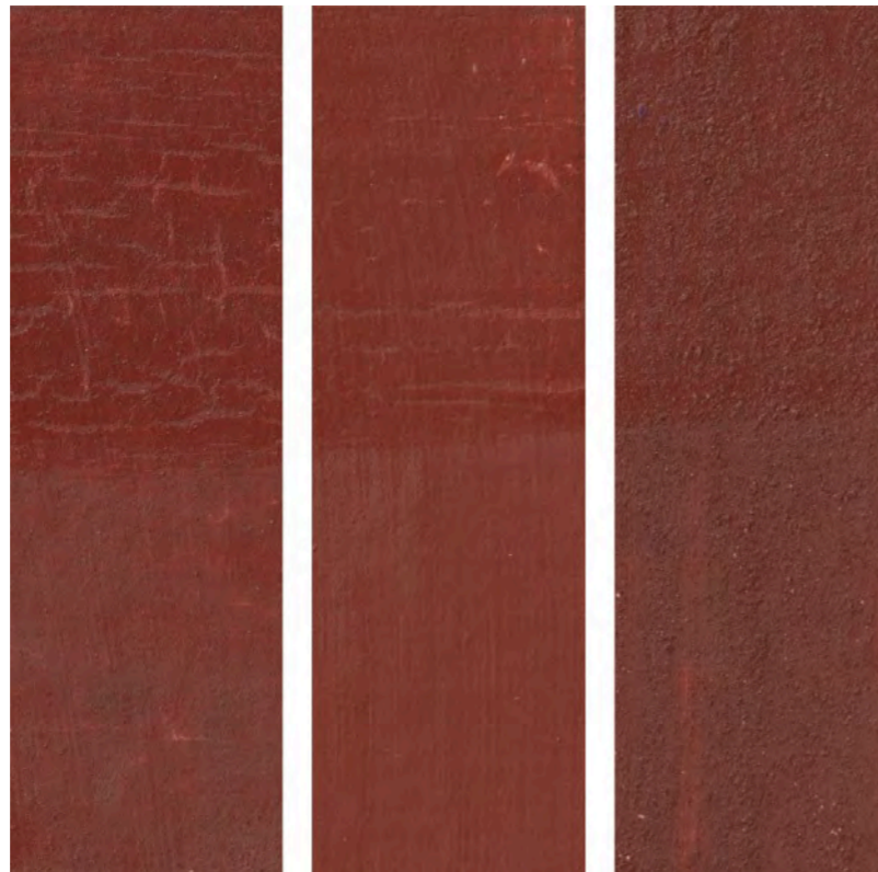
Left to right: ammonium carbonate, bicarbonate of soda and borax, with a silk glaze applied to the top half of each sample.
